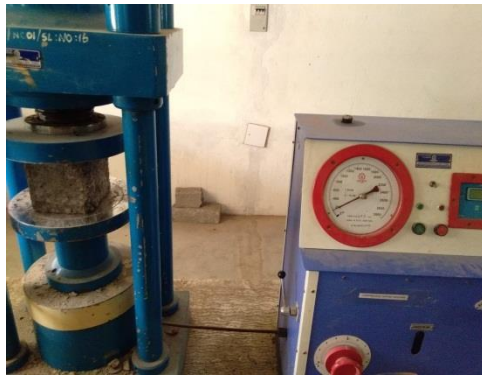
Figure.2 Testing of compressive strength
