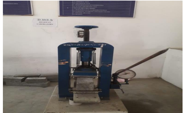
Figure.4 Testing of Flexural strength for concrete
