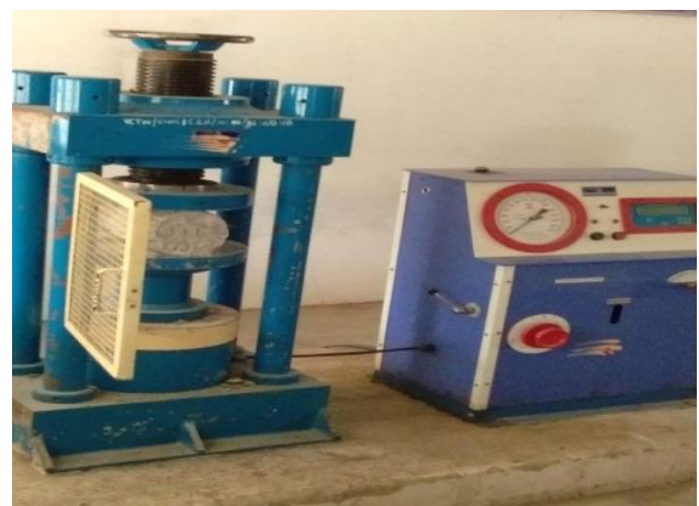
Figure.6 Testing of Split Tensile strength
